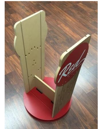
4. Line up the screw heads on the Reinforcement Panel (C) with the keyhole slot on the insides of each Side Panel (D). Once in, gently push the Reinforcement Panels (C) towards the floor until locked into place.
